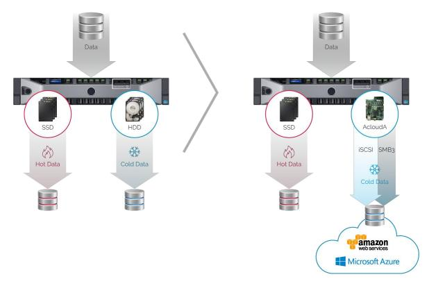
AcloudA replaces an HDD and sends data automatically to cloud
