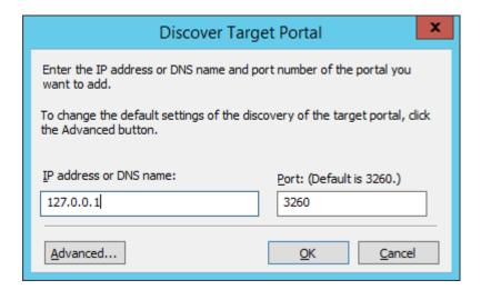
4. Click the Advanced button. Select Microsoft iSCSI Initiator as a Local adapter and select Initiator IP (leave default for 127.0.0.1). Confirm the actions to complete the Target Portal discovery.
