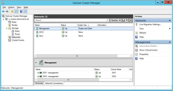
3. In the Actions tab, click Live Migration Settings. Uncheck the synchronization network, while the iSCSI network can be used if it is 10+ Gbps. Apply the changes and click OK.
