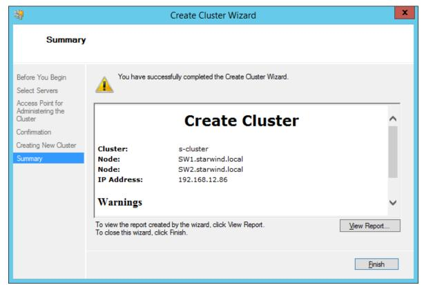
NOTE: If checkbox Add all eligible storage to the cluster is selected, the wizard will add all disks to the cluster automatically. The device with the smallest storage volume will be assigned as a Witness. It is recommended to uncheck this option before clicking Next and add cluster disks and the Witness drive manually.
