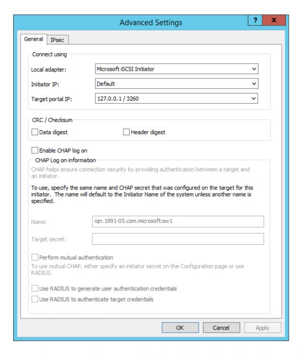
NOTE: It is recommended to connect the Witness device only by loopback (127.0.0.1) address. Do not connect the target to the Witness device from the partner StarWind node.
