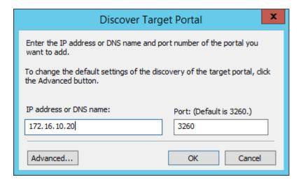
7. Select Microsoft iSCSI Initiator as the Local adapter, select the Initiator IP in the same subnet as the IP address of the partner server from the previous step. Confirm the actions to complete the Target Portal discovery.
