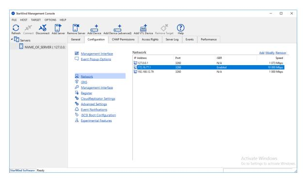
6. To enable iSER support, click on the network (here 172.16.77.1), press the Modify button and enable the checkbox Enable iSER for this Interface... in the appeared window. Click OK to confirm.
