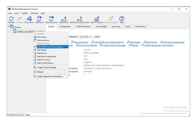
8. lick on the newly created target and press the Config... button. Enter Target Alias and port number (default is 4420) and click the Add File-Based Disk... button.
