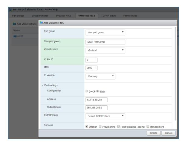
3. Add a Virtual Machine Port Groups on the vSwitch for iSCSI traffic (vSwtich1) and on the vSwitch for Synchronization traffic (vSwitch2).
