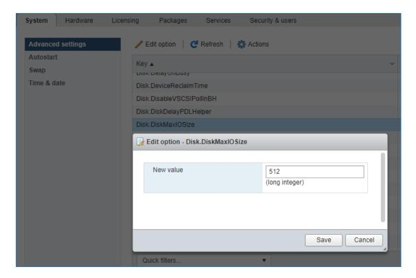
NOTE: Changing Disk.DiskMaxIOSize to 512 might cause startup issues with Windows-based VMs, located on the datastore where specific ESX builds are installed. If the issue with VMs start appears, leave this parameter as default or update the ESXi host to the next available build.
