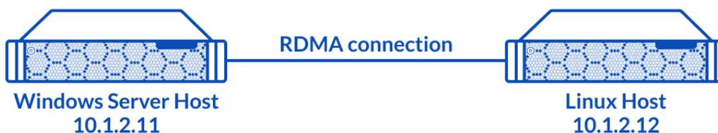
In this guide, to measure the RDMA connection between Windows and Linux operating systems, two servers are connected directly over RDMA. As an example, Windows Server 2016 has been installed on Host 1 and Linux CentOS 7 has been installed on Host 2.
