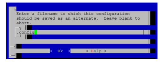
Compile the core. Use the Iscpu command to learn the number of logical CPUs in the system; use that number as the parameter in the make -j command (make-j\* where \*-
